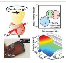
Cross-linked lysozyme crystals infiltrated with Au or Ag form a novel hybrid optical material with a strong plasmonic response. Absorption measurements of infiltrated crystals with up to 36% in weight of Au or Ag can be fitted using a distribution of isolated ellipsoidal particles, while fluorescence lifetime spectra reveal contributions from quenched protein fluorescence and characteristic emission from small Au-nanoclusters.
