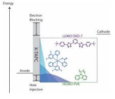
The influence of varying hole-injection and electron-blocking properties is studied using different crosslinkable hole conductors of the 4,4'-(cyclohexane-1,1-diyl)bis(N,N-dip-tolylaniline) (TAPC) family in blue phosphorescent organic light-emitting diodes (OLEDs) consisting of polyvinylcarbazole (PVK)/bis[(4,6-di-fluorophenyl)pyridinato-N,C²](picolinato) iridium(III) (FIrpic)/1,3-bis(5-(4-tert-butylphenyl)-1,3,4-oxadiazol-2-yl)benzene (OXD-7)-based solution-processed devices.
